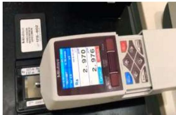
Fig 3.2 Surface roughness tester
