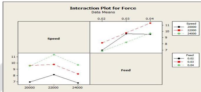
Figure 4. Interaction plot for SN ratios for Thrust Force
