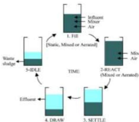
Fig -1: SBR operation for each tank for one cycle
